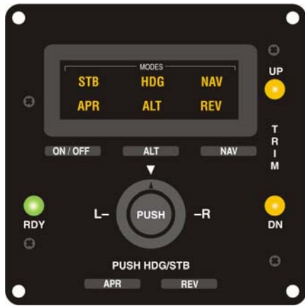
Fig. 2-10. AP Display, STB, HDG, NAV, APR, ALT, REV Annunciations Appear, TRIM UP, TRIM DN, RDY Lamps Illuminated (System Fifty)
