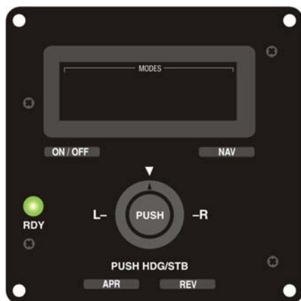
Fig. 2-3. AP Display, RDY for Operation (System Forty)
