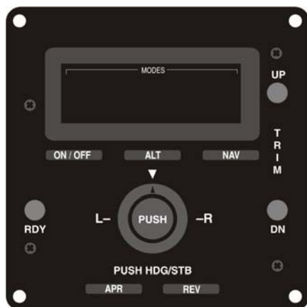
Fig. 2-16. AP Display, Turn Coordinator Failure, RDY Lamp Does Not Re-Illuminate (System Fifty)
